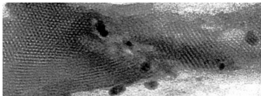
Fig. 2 TEM of the as-obtained silicate ( \times 240\ 000 ).
